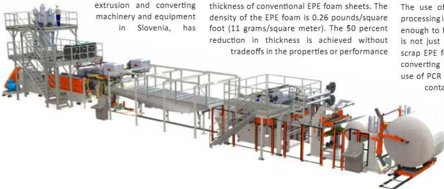
Image shows an Alemo EPE foam line configured to make 0.02-inch-thick sheet in roll widths of 95 to 120 inches—50 percent thinner than conventional EPE foam sheet. Courtesy of Alemo
